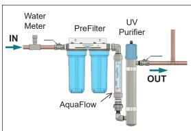
For a complete Whole House Water Treatment it is highly recommended to add a UV Disinfection system after the Descaler for top water quality and peace of mind.
